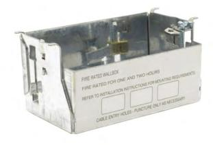
The Voltex Fire Rated Wall Box is designed for mounting switches and outlets in walls that have a specified Fire Rating. Fully compliant to Australian Standards. Tested to 1 and 2 hour Fire Rating in single and back-to-back installation. Comes complete with intumescent pads and acoustic seal.
